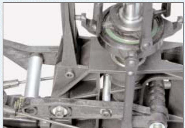
Swashplate linkage incorporating reinforced collective pitch bridge
