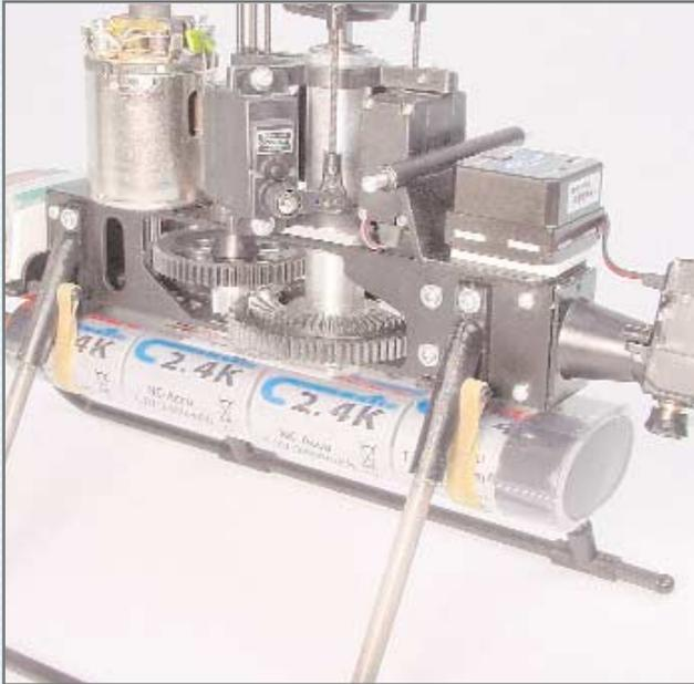
The torsional rigidity of the chassis is exceptionally high, as it is machined from an aluminium square-section profile. The chassis includes pre-cut openings for the tail boom support, skid landing gear and front structure. Aluminium dome support; tail boom bracket and front structure made of glass fibre reinforced plastic.
